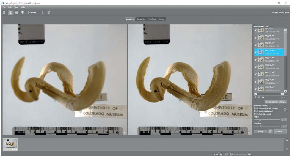
Figure 7. Helicon Focus interface. The left pane displays a selected source image (UCM 58908 Hydrophis platurus ) in the stack with only the upper midbody in focus. The right view shows the fully focused output image that was rendered using Method B (depth map) to combine all 20 source images.
