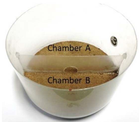
Figure 1. The two-chambered test arena for video tracking experiments with Porcellio scaber . Animals could select between uncontaminated (chamber A) and pyrethrin-contaminated soils (chamber B).
