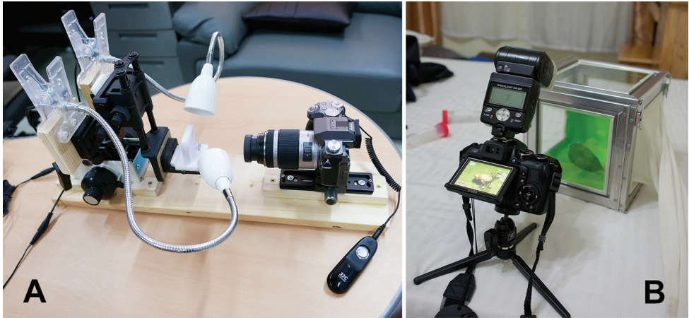
Figure 11. Macro photography setups for multi-day collecting trips. A A simple handmade collapsible macro-photography unit for focus stacking B A setup for photographing live tephritid flies. Please see the Materials and methods for details of the camera setups.
