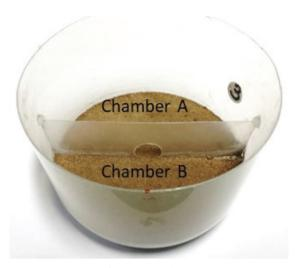
**Figure 1.** The two-chambered test arena for video tracking experiments with *Porcellio scaber*. Animals could select between uncontaminated (chamber **A**) and pyrethrin-contaminated soils (chamber **B**).
