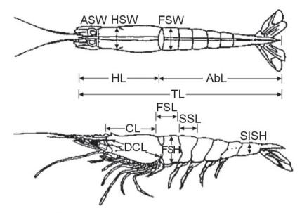
**Figure 3.** Diagram of a shrimp showing the body segments measured (Tzeng et al. 2001): total length (TL), antennal spine width (ASW), hepatic spine width (HSW), cephalothorax length (CL), diagonal cephalothorax length (DCL), first abdominal segment length (FSL), first abdominal segment width (FSW), first abdominal segment height (FSH), second abdominal segment length (SSL), sixth abdominal segment height (SISH), abdomen length (AbL) and head length (HL).
