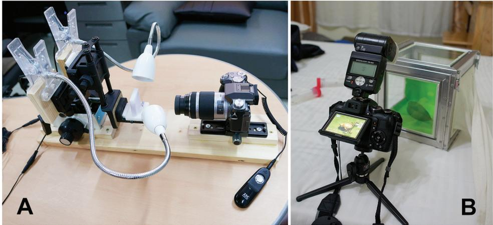
**Figure 11.** Macro photography setups for multi-day collecting trips. **A** A simple handmade collapsible macro-photography unit for focus stacking **B** A setup for photographing live tephritid flies. Please see the Materials and methods for details of the camera setups.
