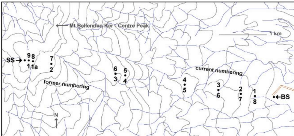
**Figure 2.** Plan of the Mt Bellenden Ker cableway showing current and former tower numbers. SS = summit station, BS = base station. Contours (100 m) and streamlines are only approximate and are from the 1:50000 scale 'Bartle Frere' map produced by the Royal Australian Survey Corps in 1986.
