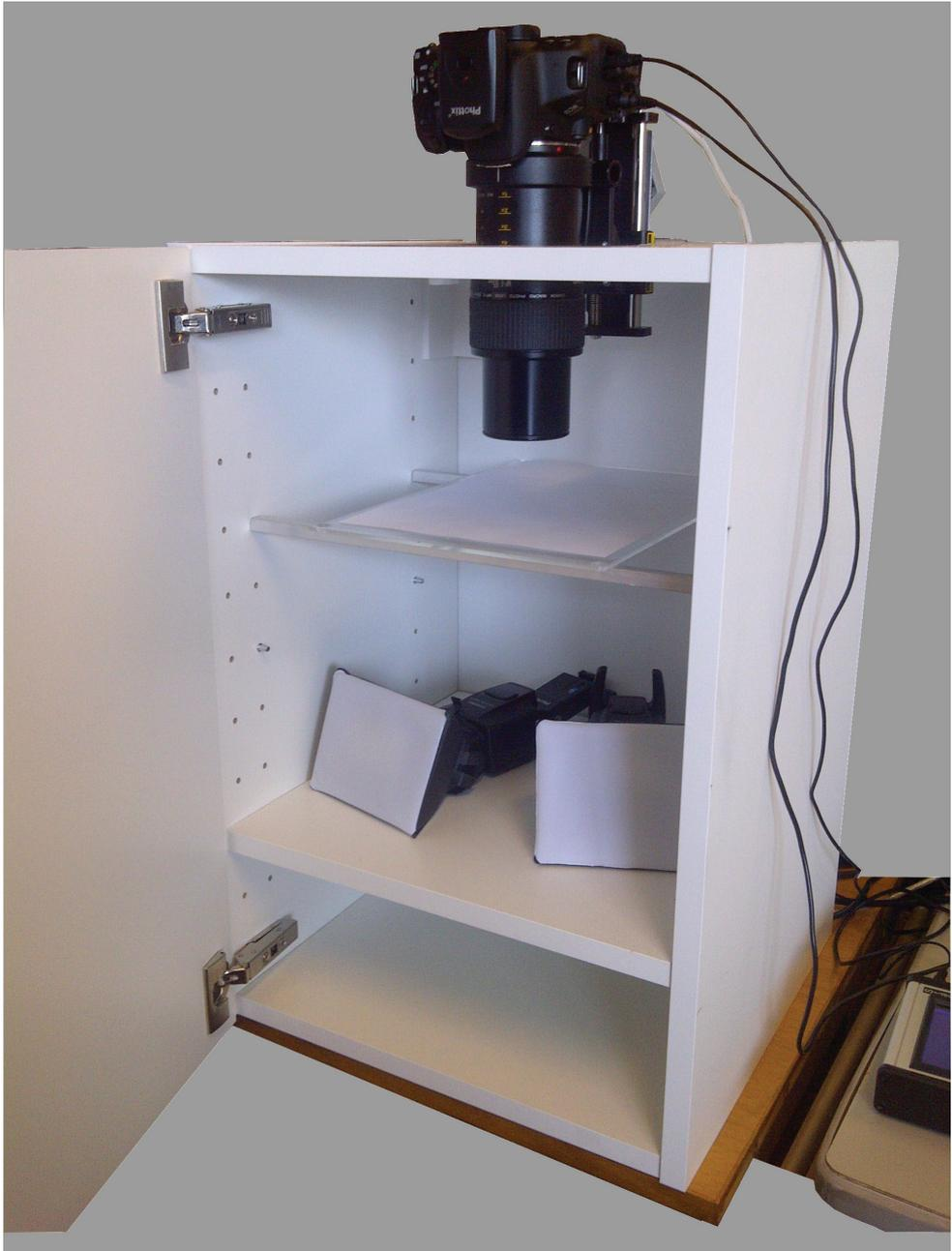
**Figure 1.** The Canon-Cognisys set-up at the RBINS. The Canon 600D Camera, equipped with a Canon MP-E 65 mm 1:2.8 1–5× Macro Photo Lens, is mounted on the vertically positioned StackShot (Cognisys inc.). In the Ikea closet, at the bottom, you see the two Yongnuo YN560-II speedlights positioned frontally and above is the plexiglas plate covered with paper to position the specimen.
