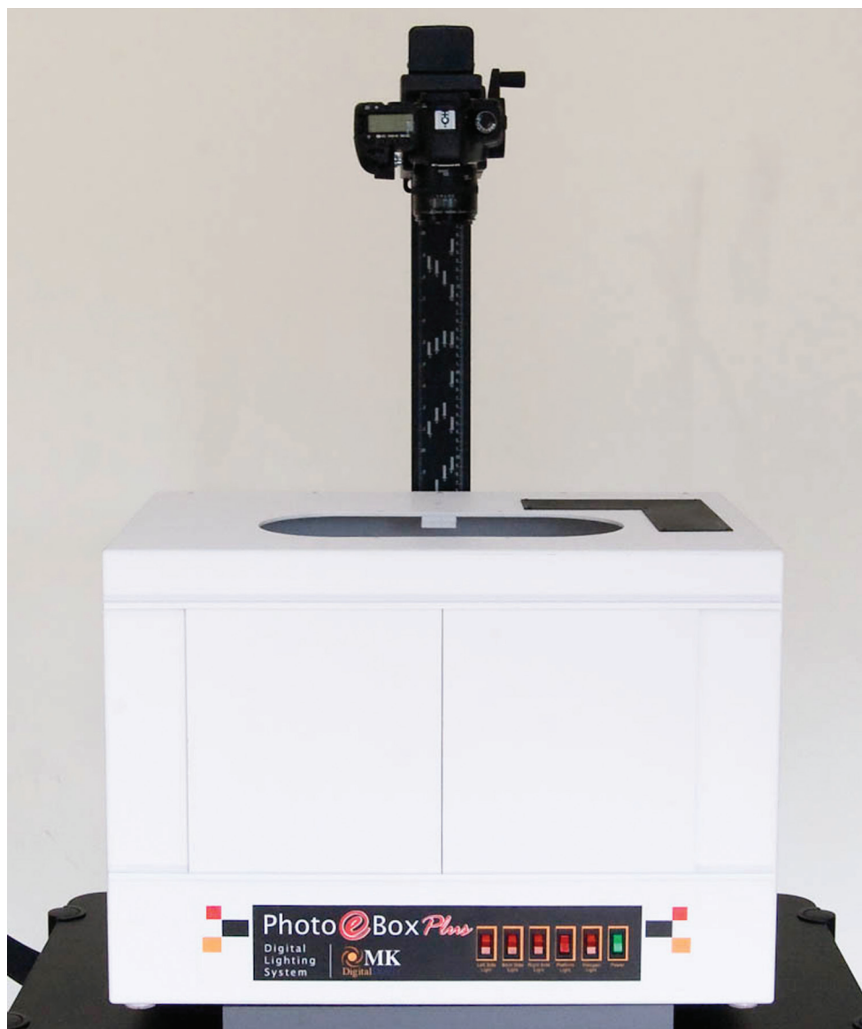
Figure 2. NYBG imaging station consisting of a Canon Eos 5D Mark II digital camera body, a Canon EF 50mm f/2.5 Macro lens, Photo e-Box Plus 1419 from MK Direct, and Kaiser RS 1 copystand.
