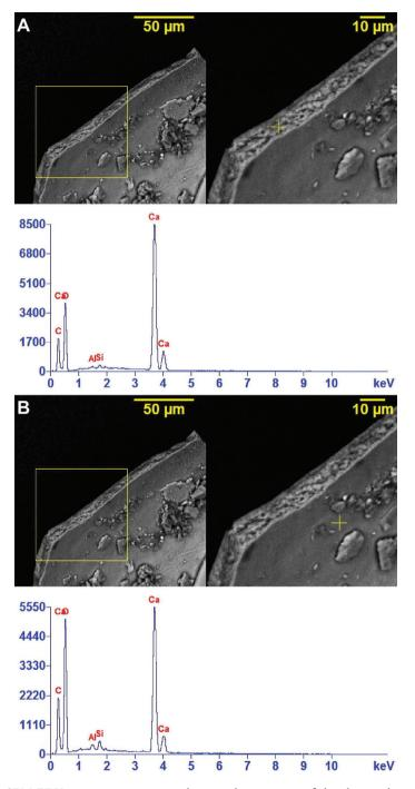
**Figure 10.** SEM-EDX spectroscopic images showing the spectrum of the elemental content in two regions of the inner shell of *K. nodongense* sp. n. paratype (NMBE 534361/2). **A** surface of shell edge **B** the inner layer of the shell. Both regions (yellow +) show the presence of calcium (Ca), aluminum (Al), silicon (Si) and carbon (C).
